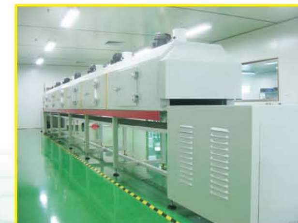
Electric heating tunnel furnace
