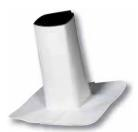
Fabricated using 60-mil reinforced Sure-Weld® and Sure-Flex™ membrane, square tubing wraps are designed to flash square metal tubing. A split and overlap tab are incorporated into these parts to allow the flashings to be opened and wrapped around a square penetration with an obstruction. Other sizes and colors available through special order.
