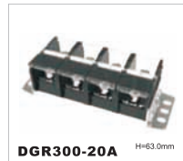
DGR300-20A H=63.0mm CE 1000V/300A 150mm 2 UL 600V/300A 20-300kcmil Poles 1P-XXP
