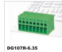
DG107R-6.35 CE 600V/32A 0.5-4.0mm 2 UL 300V/30A 20-10AWG Poles 1P-XXP
