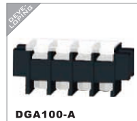
DGA100-A IEC 800V/101A 35mm 2 UL 600V/101A 20-2AWG Poles 1P-XXP
