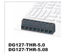
DG127-THR-5.0 DG127-THR-5.08 CE 250V/15A 0.2-1.5mm 2 UL 300V/12A 26-14AWG Poles 2P,3P-24P
