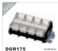
DGR175 H=48.0mm IEC 800V/175A 70mm 2 UL 600V/175A 20-2/0AWG Poles 1P-XXP
