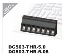
DG503-THR-5.0 DG503-THR-5.08 IEC 250V/18A 2.5mm 2 UL 300V/10A 24-12AWG Poles 2P,3P-24P
