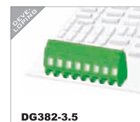
DG382-3.5 IEC 130V/12A 1.5mm 2 UL 250V/10A 30-14AWG Poles 2P,3P-24P
