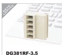
DG381RF-3.5 IEC 160V/8A 1.5mm 2 UL 150V/8A 26-16AWG Poles 3P-5P
