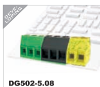
DG502-5.08 IEC 250V/18A 2.5mm 2 UL 300V/10A 24-12AWG Poles 2P,3P-24P
