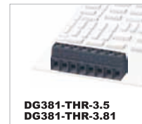
DG381-THR-3.5 DG381-THR-3.81 CE 130V/10A 0.2-1.0mm 2 UL 150V/10A 30-16AWG Poles 2P,3P-24P
