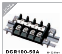
DGR100-50A H=50.5mm IEC 800V/100A 35mm 2 UL 600V/101A 20-2AWG Poles 1P-XXP
