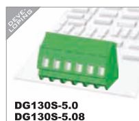
DG130S-5.0 DG130S-5.08 IEC 250V/20A 2.5mm 2 UL 300V/20A 26-12AWG Poles 2P,3P-24P
