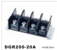
DGR200-20A H=58.0mm CE 1000V/200A 95mm 2 UL 600V/200A 20-4/0AWG Poles 1P-XXP
