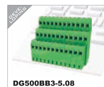
DG500BB3-5.08 IEC 250V/18A 2.5mm 2 UL 300V/10A 24-12AWG Poles 3*(2P,3P-24P)
