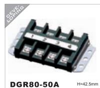
DGR80-50A H=42.5mm IEC 800V/80A 25mm 2 UL 600V/80A 20-4AWG Poles 1P-XXP
