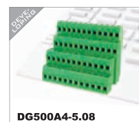
DG500A4-5.08 IEC 250V/18A 2.5mm 2 UL 300V/10A 24-12AWG Poles 4*(2P,3P-24P)
