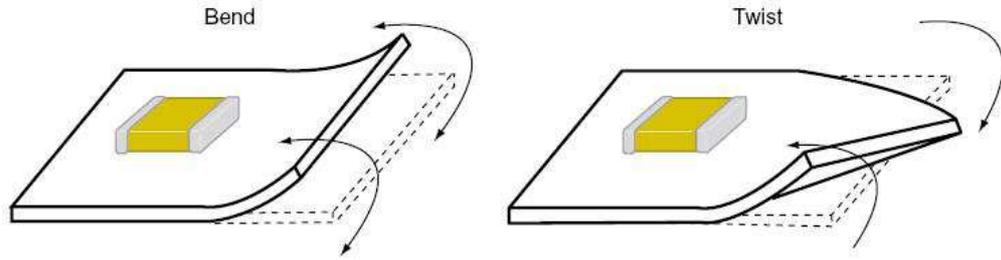
2) When functional check of the P.C. board is performed, check pin pressure as it tends to be adjusted higher for fear of loose contact. If the pressure is excessive and bends the P.C. board, it may crack the chip capacitor or peel the terminations off.
