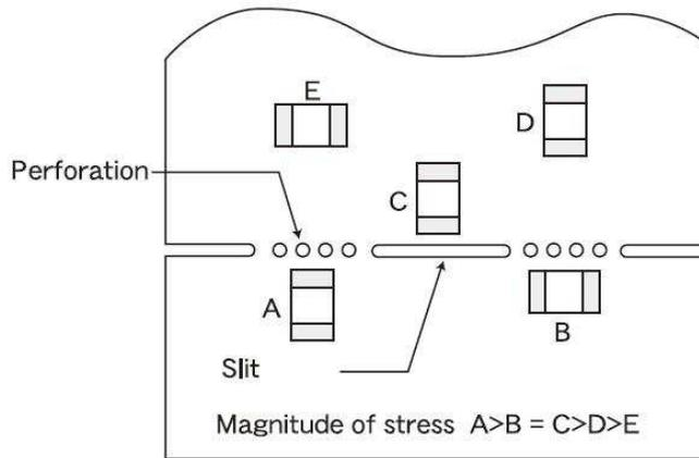
5) Recommended chip capacitor layout is as follows:
