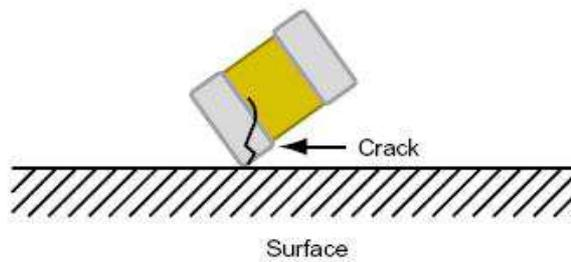
2) Avoid piling up P.C. boards after mounting. The corner of the P.C. board may hit the chip capacitor of another board causing the chip to crack or dislodge.
