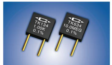
The Tetrinox® Resistance System was introduced by Caddock in 1975. Tetrinox provides a wide range of resistivities, with the higher resistivities capable of producing resistance values up to 100 times higher than other ultra-low TC resistors in a similar size component. The essentially linear TC is well within 10 ppm/°C over the entire temperature range from -55°C to +125°C. By using TK resistors engineers can design high precision circuits with lower current drain and lower power requirements.
