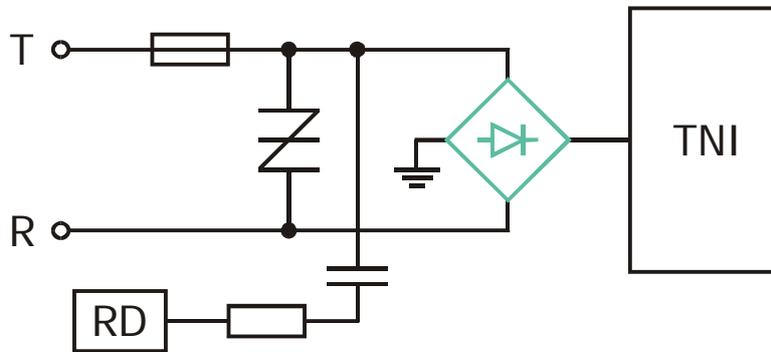
Rectifier bridges are commonly used in telecommunications equipment, such as Analogue Line Cards, Customer Premises Equipment (CPE – phones, modems, faxes and PABX), High Speed Transmission equipment such as ADSL, SHDSL, ISDN or E1/T1. Rectifiers can be used as clamping / steering diodes or to build common protection among multiple lines.
