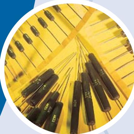
Our wirewound resistors feature an alloy resistance wire precision-wound to a heat-conducting ceramic substrate, with welded endcaps and lead terminations, and silicone conformal coating protecting the resistive element.
