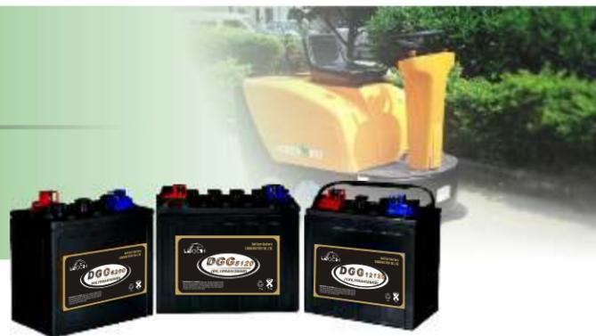
DGG Series batteries are valve regulated, rechargeable lead-acid batteries which, in contrast to conventional systems, retain the electrolyte is gel and also are using of tubular plates to increase cycle life by preventing of material shedding and pressing of PAM specially in discharged state.
