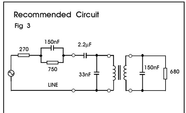
In practice, the 600Ω load resistor will connect to a low output impedance TX driver. The 150nF capacitor should appear in parallel with the 680Ω load resistor (rather than in parallel with transformer winding) to obtain optimum TX flatness to line.
