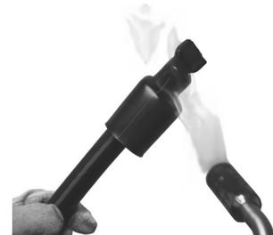
2. Beginning at closed end apply heat, blue thermochromatic lines will begin to disappear at 150° C. Gradually, move heat source to open end and around cap. Once lines are no longer visible and adhesive flows out of open end, discontinue heating.
