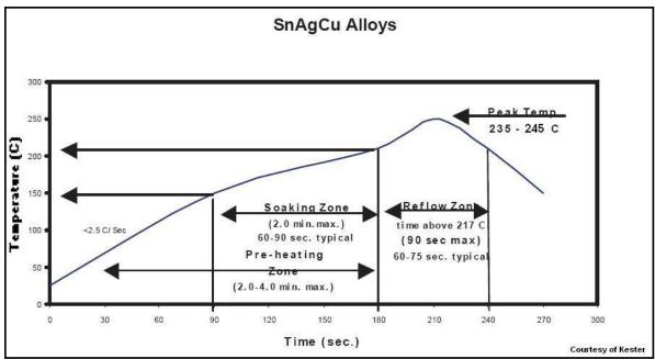
Customer will carefully select the final soldering thermal profile. The thermal profile depends on the choice of the solder paste, thickness and color of the carrier board, heat transfer and size of the penalization.
