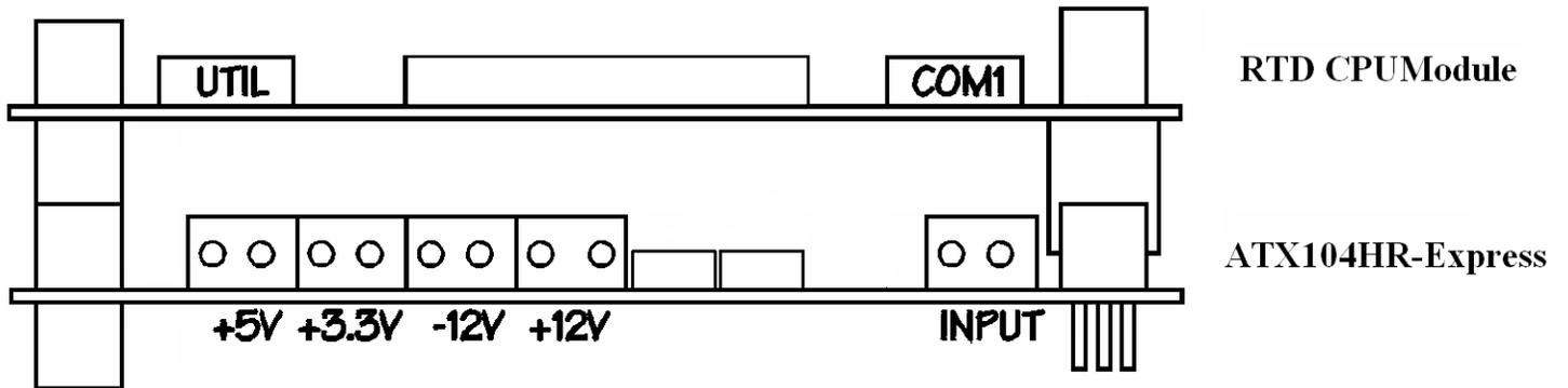
**Figure 3: ATX104HR-EXPRESS powering an RTD PC/104-EXPRESS cpuModule stack. PCI bus shown with non-stack through connector. Standard is press fit stack through.**
