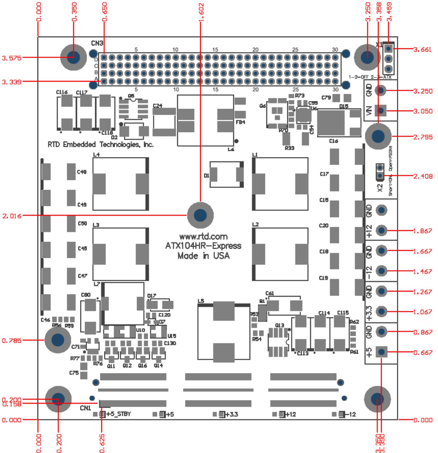
Figure 6: Dimensioned Drawing
