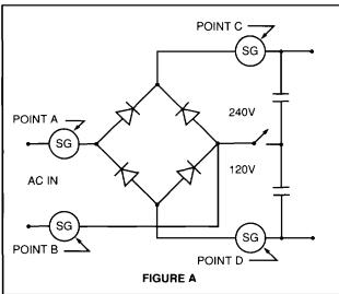
If the resistance of one Surge-Gard does not provide sufficient inrush current limiting for your application, two or more may be used in series or in separate legs of the supply circuit. Surge-Gards cannot be used in parallel since one unit will tend to conduct nearly all the current available. Surge-Gards may be used in the AC (Point A or B) or the DC (Point C or D) locations in the circuit.
