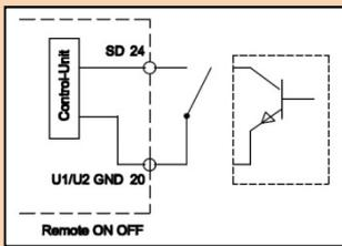
Enable a 10...30Vdc 20mA voltage signal to (Rmt/Rm) to shutdown the HPW, the yellow LED lights and 0V is distributed to the outputs. If the shutdown is short circuited or <math><500mV</math> are applied to (Rmt/Rm), the HPW „tickers“, the yellow LED flashes and 5V is distributed to the outputs. Disable the remote voltage to restart the PSU
