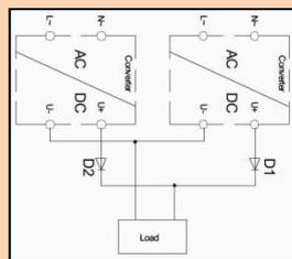
To increase system availability up to five HPW can be used in parallel operation mode. Please make sure that wiring length from all units to the load is equal. Full redundant operation modes require external diodes. We suggest to use our RED00202 DIN-Rail N+1 redundant module für professional redundancy.
