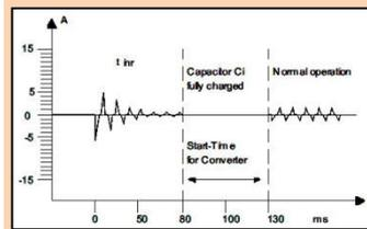
While connecting the HPW to the AC wire network its inrush current is limited to <math><7A</math> (typ.). The start capacitors are loaded after 80ms and the HPW actuates. After passing softstart (active PFC) the power supply is ready for operation after a total of  $t=130ms</math>.$
