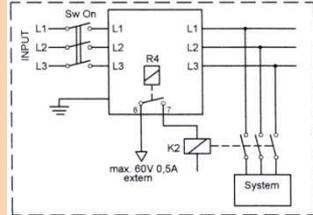
In case of phase loss relay 4 opens after a delay time of 30ms. Synchronistic the relay of the appropriate phase opens, too and its green LED extinguishes. When the phase sequence is incorrect, relay 4 opens after a delay time of 30ms. The Phase Error LED lights red. When the phase sequence is correct the LED is off and the relay 4 is closed.
