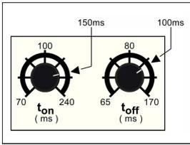
The Ton-time (limiting period) and the Toff-time (response time to arm the circuit after a phase lost or voltage drop) can be adjusted by the owner. The factory settings are Ton=150ms and Toff=100ms. Note: the adjusting range is non-linear.
