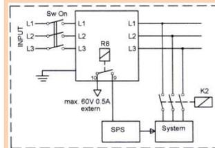
The asymmetry monitoring detects a voltage difference of the three phases to each other. This kind of measuring enables work without the N line (four wire system). If the voltage of the measured AC line drops or exceeds 15% of its nominal selected input relay 8 opens 8-10s delayed and the Asymmetry LED lights red. Measuring tolerances are  $\pm 2\%$ .
