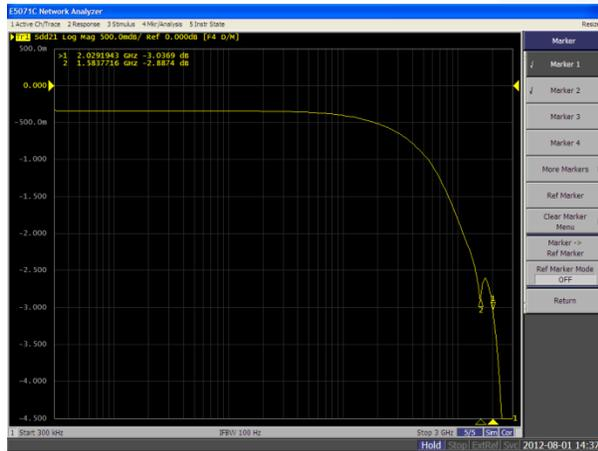
Figure 17. MHL Path SDD21 Insertion Loss Curve
