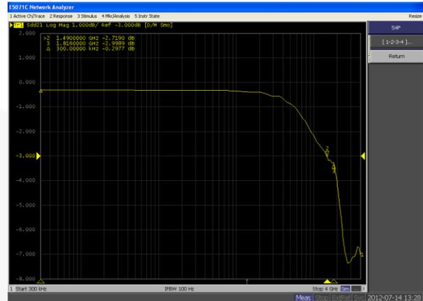
Figure 18. USB Path SDD21 Insertion Loss Curve
