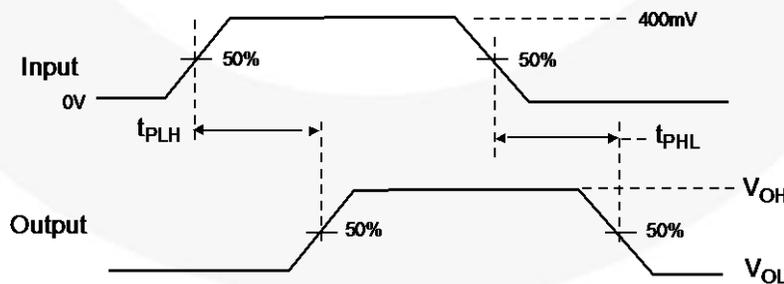
**Figure 9. Propagation Delay ( $t_{RtF} = 500ps$ )**
