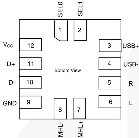
Figure 3. Pin Assignments
