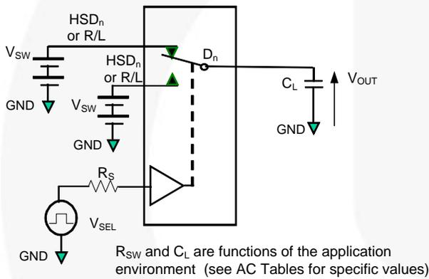
$R_{SW}$  and  $C_L$  are functions of the application environment (see AC Tables for specific values)
