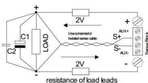
**Remote Sensing (2V per lead load, fig6)**
