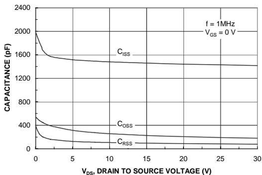
Figure 8. Capacitance Characteristics.
