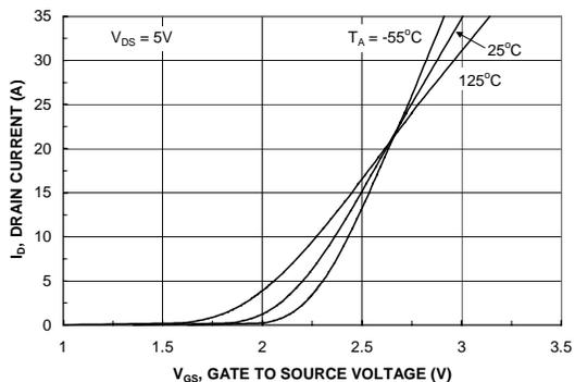
Figure 5. Transfer Characteristics.
