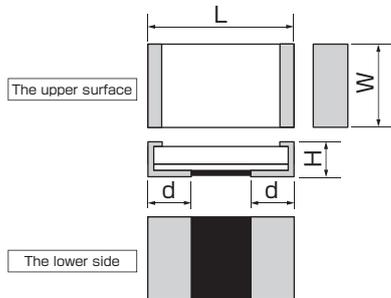
Rated resistance value is marking with 4-digit on the over coating.
