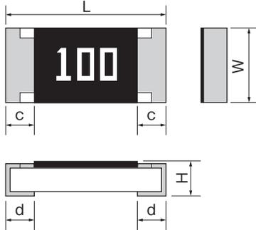
Rated resistance value is marked with 3-digit on the over coating
