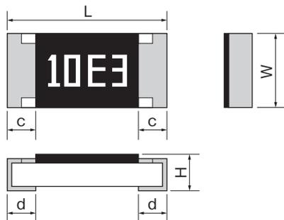
Rated resistance and T.C.R. value are marked with 4-digit on the over coating.
