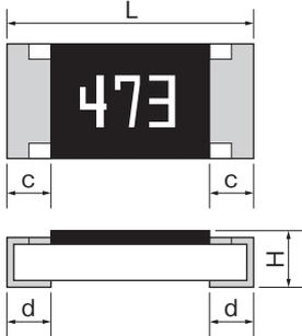
Rated resistance value marking is with 3-digit (E24) or 4-digit (E96) on the over coating.
