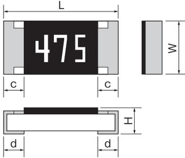
Rated resistance is marked with 3-digit(E24) on the over coating.
