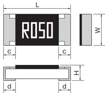
Rated resistance is marked with 4-digit on the over coating. (RLC20~RLC63)
