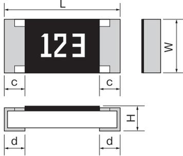
Rated resistance value is marked with 3-digit on the over coating.
