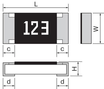
Rated resistance value is marked with 3-digit (E24) on the over coating except 4-digit (E96).
