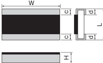
Rated resistance is marked with 4-digit on the over coating.
