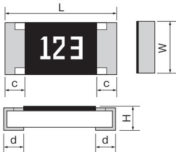
Rated resistance is marked with 3-digit (E24) or 4-digit (E96) on the over coating.
