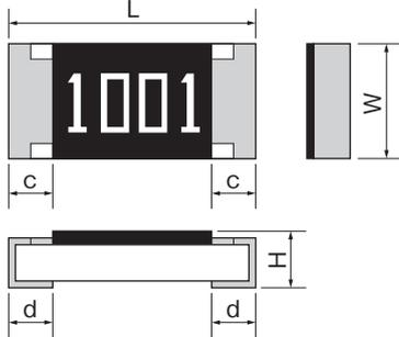
Rated resistance value is marked with 3-digit (E24) or 4-digit (E96) on the over coating.
