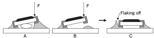
7.6 The overcoat and the main body may be chipped off when you hold the parts strongly with tweezers.
