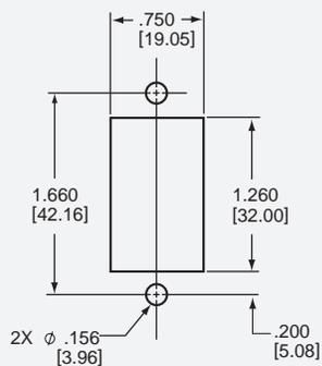
Panel Mounting Detail: Tolerance  $\pm .005$  [.13] unless noted.
