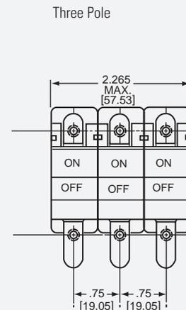
Panel Mounting Detail: Tolerance ±.005 [.13] unless noted.
