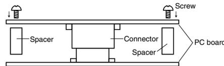
When connecting PC boards, take appropriate measures to prevent the connector from coming off.
