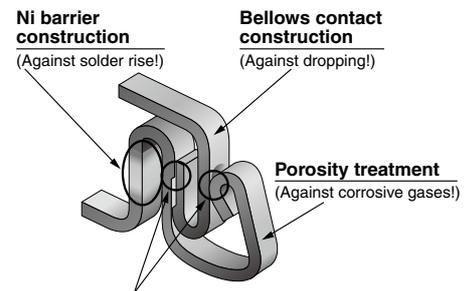
**V notch and Double contact constructions**
