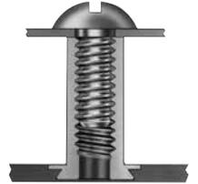
**blind:** Have closed ends that limit screw penetration and are useful for protecting internal components from damage by inadvertent insertion of extra long screws. Threads are also protected from damage and foreign matter.
