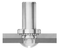
**right angle:** Provide you with strong right angle attachment points in sheets as thin as .040"/1mm. These fasteners are a cost-effective replacement for: bent edge tabs; bent center tabs; bent flanges; angle brackets; tack welds; and loose hardware.
