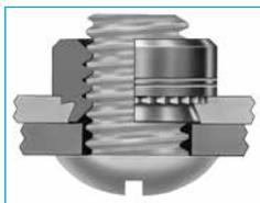
*Finally, install the mating piece from the side opposite the head of the fastener.*
