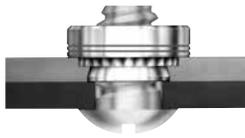
**studs and pins:** Threaded and unthreaded fasteners which are used where the attachment must be positioned before being fastened.
