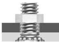
**spacers & standoffs:** Used where it is necessary to stack or space components away from the panel. Thru-threaded or blind types are generally standard.
