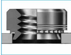
*First, insert the shank or pilot of the fastener squarely into a previously punched or drilled hole.*
