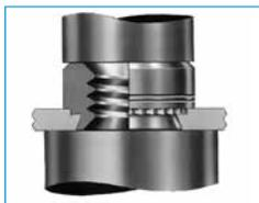
*Next, apply force until the head of the nut contacts sheet. Some types of fasteners will be fully installed when the head is flush within the sheet.*
