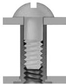
**flush fasteners:** When installed, these fasteners are completely flush within the sheet.
