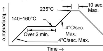
**DIP Soldering (Wave Soldering)**
