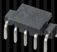
Standard header with custom bent pins and pick-and-place pad
