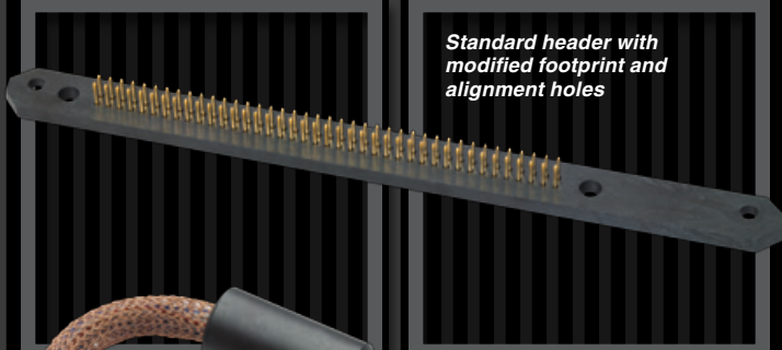
Standard header and standoffs mounted to FR4 substrate
