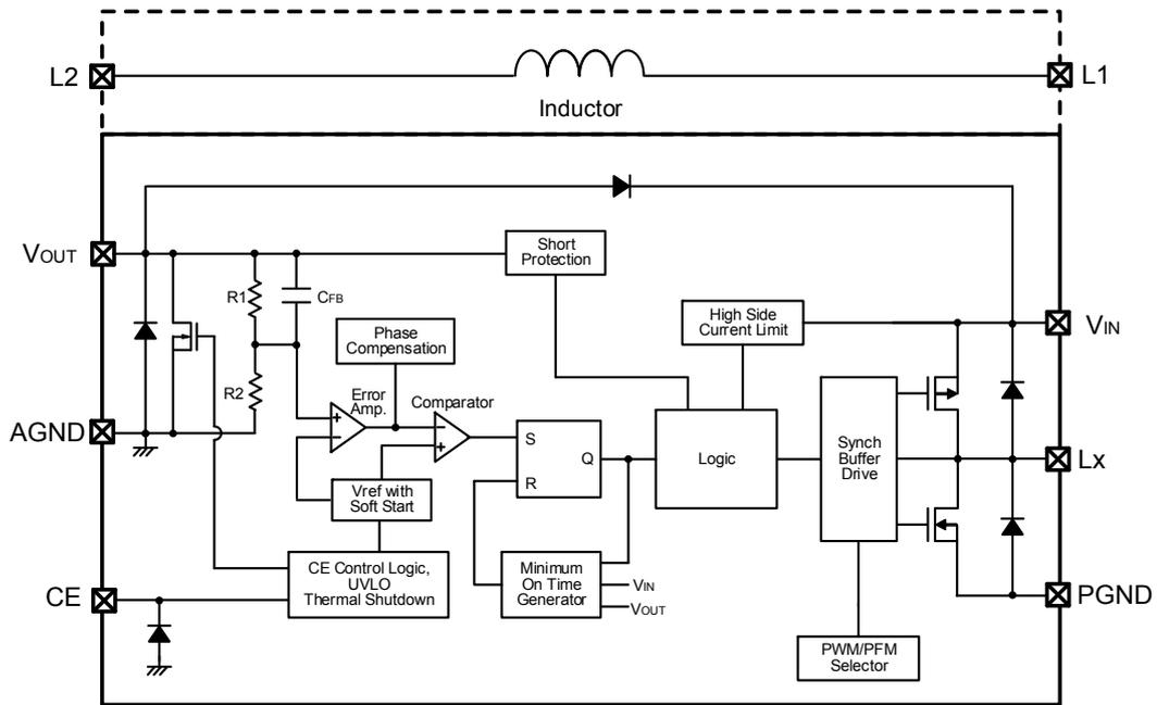
\* The XCL221 offers a fixed PWM control, a Control Logic of PWM/PFM Selector is fixed at "PWM" internally.
