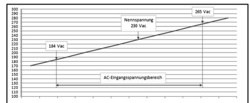
Low voltage detection  $U < 184 \text{Vac} / T_{off} > \Delta t$
