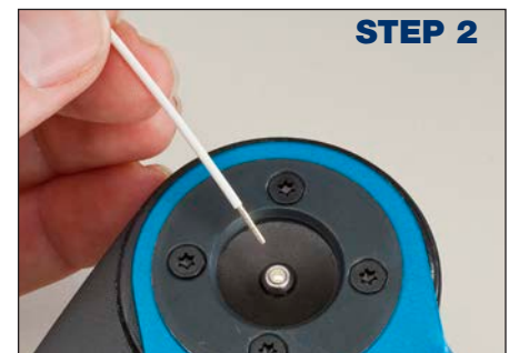
INSERT PRE-STRIPPED WIRE
