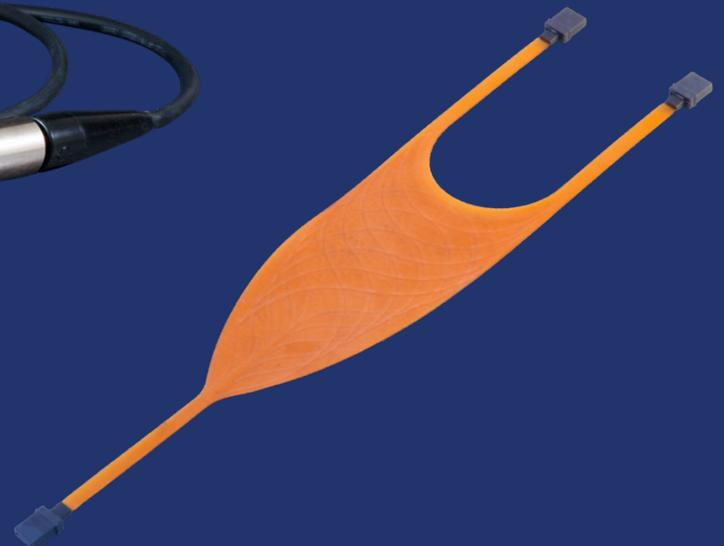
Turnkey Optical Flex circuit assembly with rugged MT ferrule terminations
