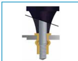
STEP 3 The pull-up stud retracts and bulges the unthreaded portion of the fastener shank against the flat undersurface.
