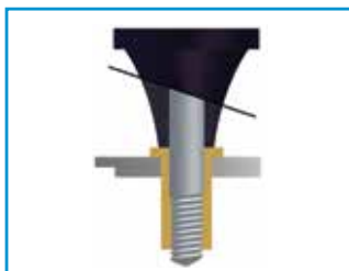
STEP 2 The fastener, on the pull-up stud, is inserted into the drilled or punched hole.
